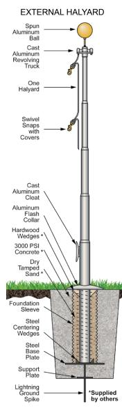
**Finish:** All of our steel flagpoles are mechanically cleaned and chemically etched to provide a smooth surface. Two coats of two-part polyurethane primer are applied before application of two polyurethane finish coats. Specify custom or one of these standard colors: Aluminum (silver), Light Bronze, Medium Bronze, Dark Bronze, Black or White. Trucks are finished to match flagpole shaft.
